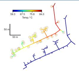
Simulated heat distribution in local district heating network: Technische Werke Ludwigshafen. Entry forward flow temperature 84*C*, backward flow temperature 60*C*.
